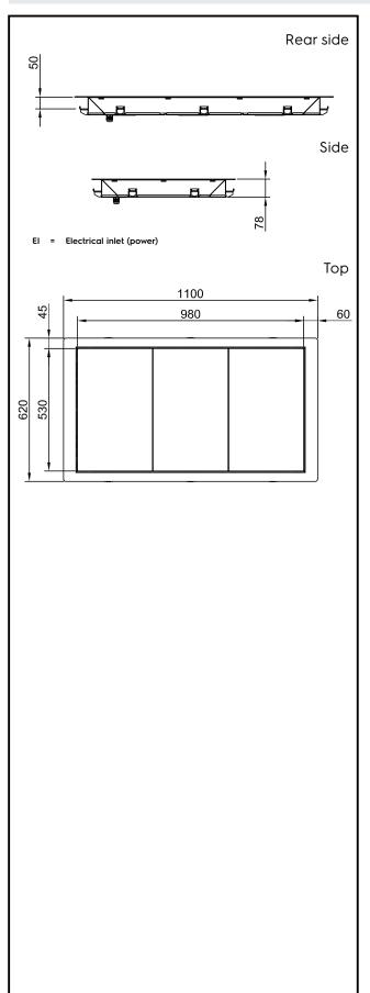
Drop-In Drop-in tempered glass top (3 GN container capacity)
