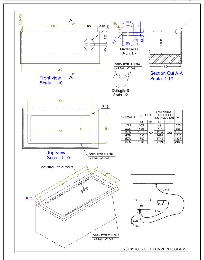
Drop-in tempered glass top (3 GN container capacity)
